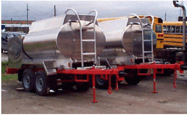
Specially designed pup trailers with a payload of 500 imperial gallons each.
